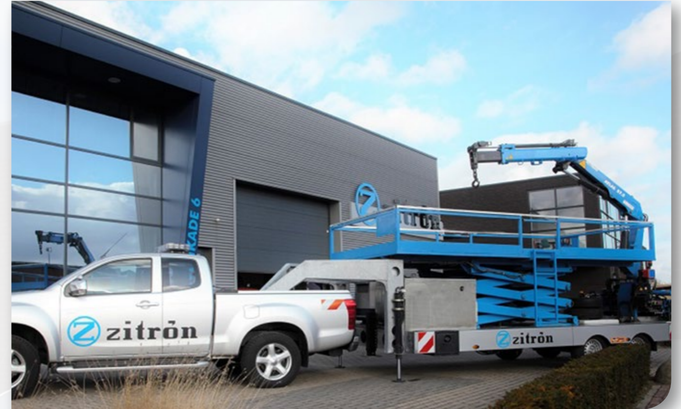
Fifth wheel Pick-up truck for dismantling, installing and inspecting jet fans
