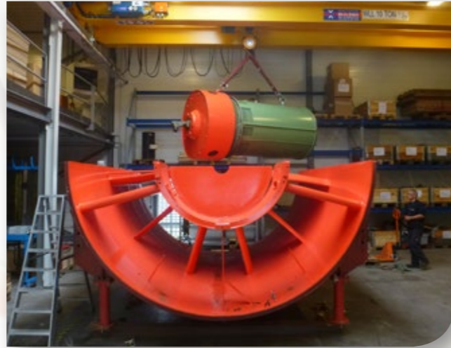
Mounting of drive motor with impeller hub in fan-motor-unit
