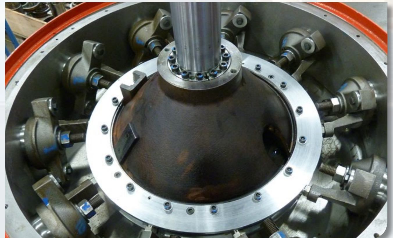
Overhauled impeller hub with blade adjustment
