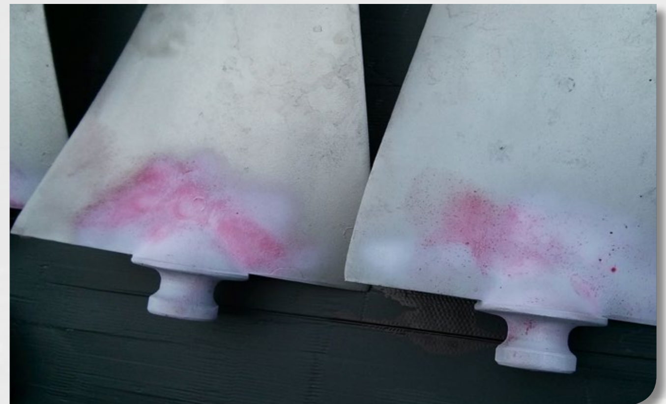
Dye penetrant test of the blades
