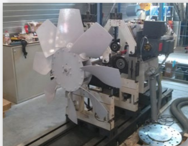
Balancing of the overhauled impeller on our proprietary balancing machine
