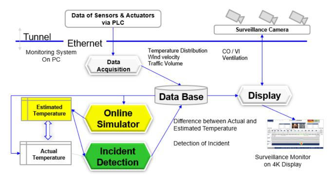
Automated incident detection by a platform approach, "model reference"
