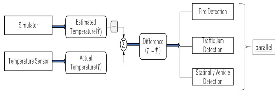
Basic principle of automated incident detection method by model reference
