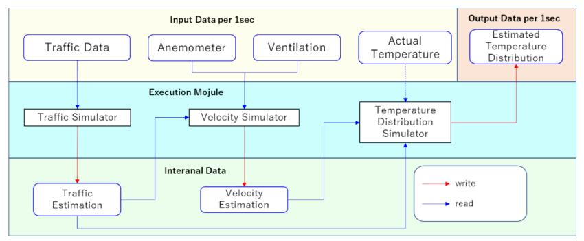
$$\frac{\partial T}{\partial t} + \frac{\partial (TV_r)}{\partial x} = D_K \frac{\partial^2 T}{\partial x^2} + \frac{\xi_T}{C_p}$$
