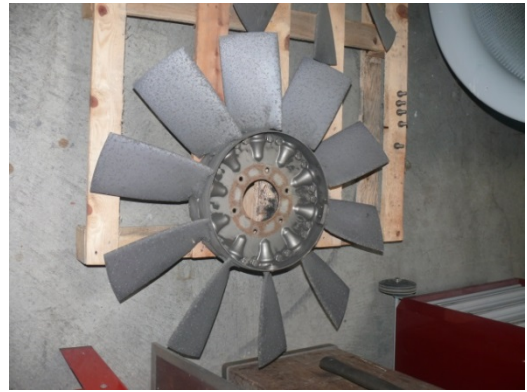
Fig 2: undamaged wheel of a jet fan
