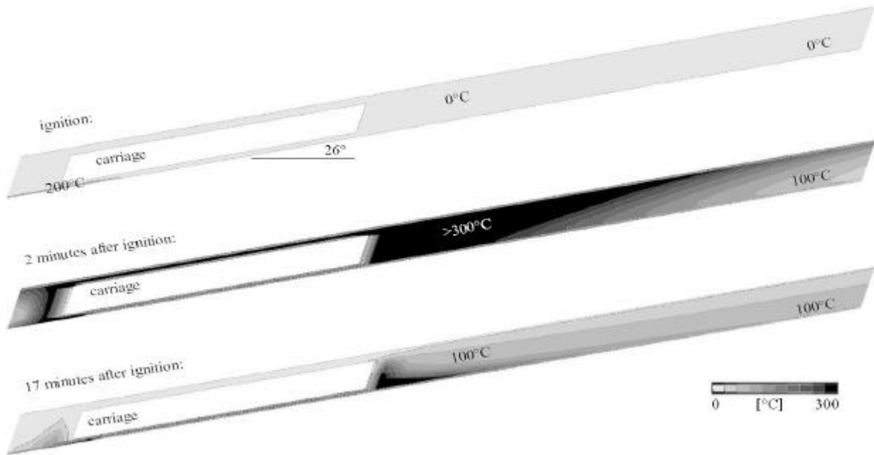
Figure 10: Temperature distribution of a tunnel fire (3300 m length, 50% gradient, 3 MW heat release)
