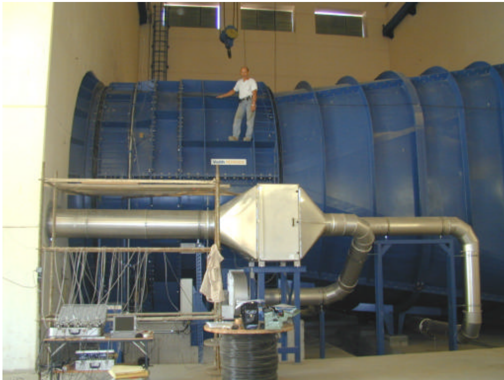
Fig. 3 NT2 Supply fan during acceptance tests
