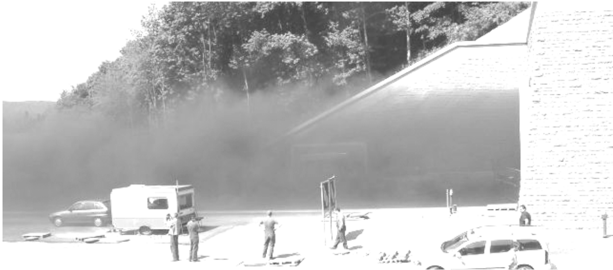
Figure 3: Smoke exhaustion from the south portal in test no. 3
