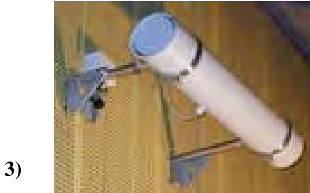
Fig. 3) A heat-transport sensor for use in road tunnels (..... http:// www.jes-et.at )
