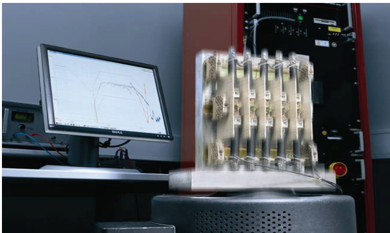
Pict. 4: Vibration Test with Stud Terminals!!
