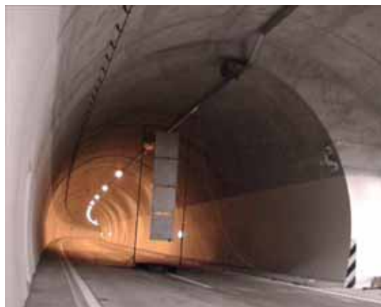
Fig. 6: Plates with temperature sensors (T1 – T5)
