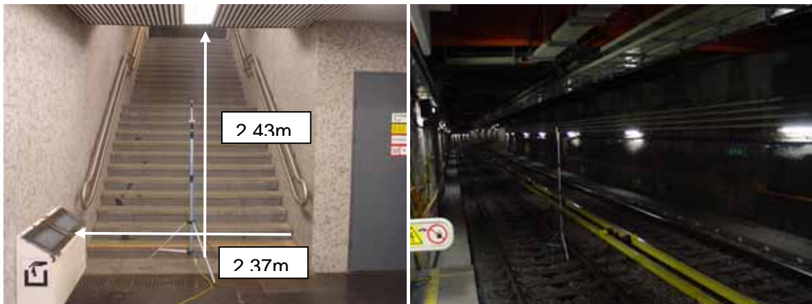
Fig. 12: Measurement arrangement entrance (left) tunnel (right)
