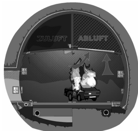
Figure 11: Cross section and damper
