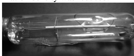
Figure 8: Melted lamp during normal operation
