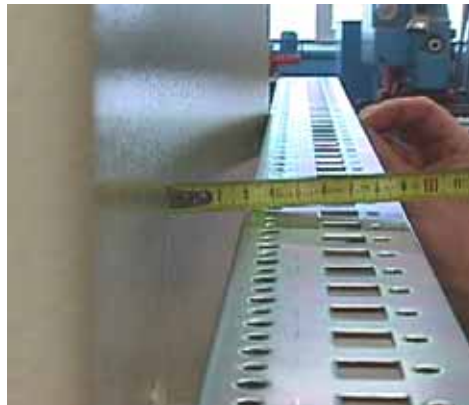
Figure 13: Displacement of a non-reinforced door at 20mbar underpressure
