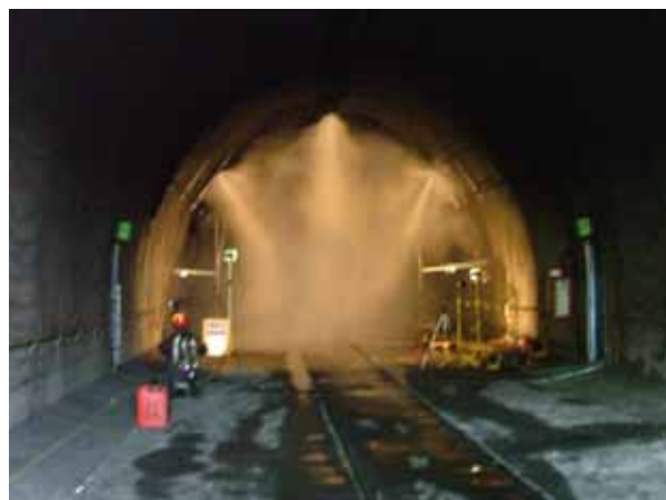
Figure 2: Test of a water mist system (Fogtec), conducted within the UPTUN Research Project
