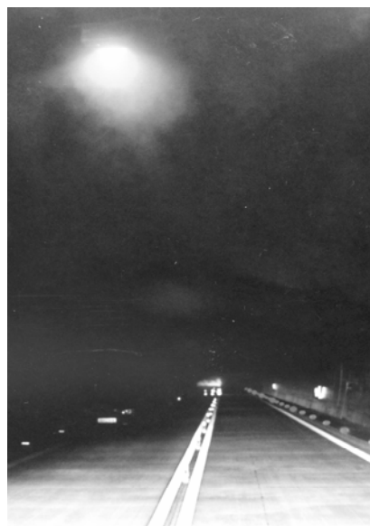
Figure 9: Visibility of the LEDs in a smoke filled tunnel
