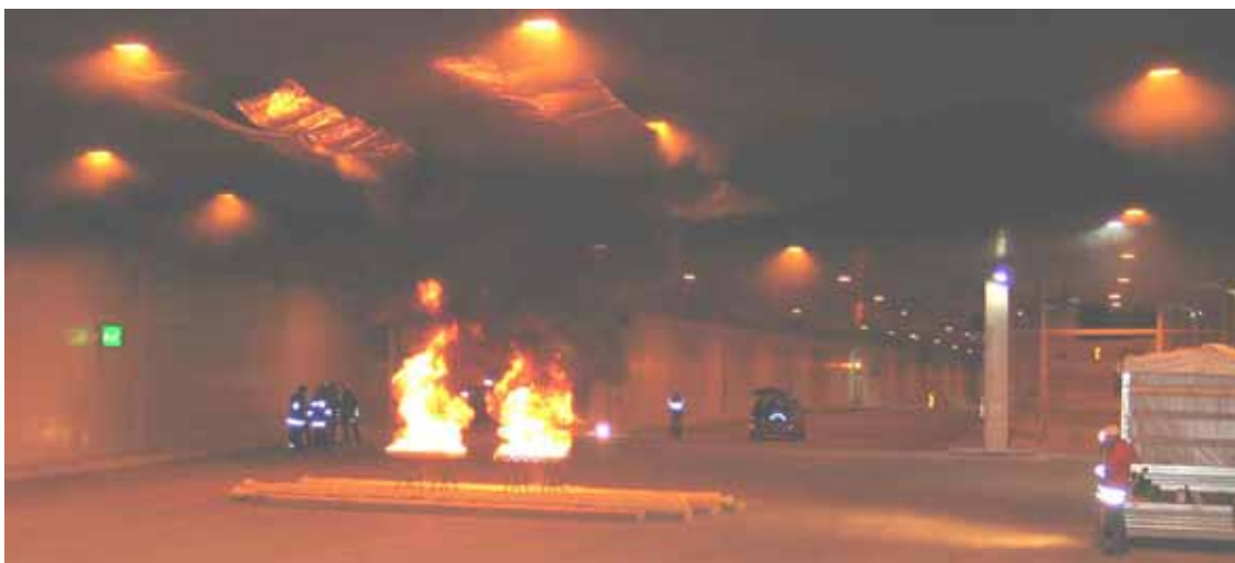
Figure 7: Test fire section I (north) with the open Muldenstraße ramp (right hand side)
