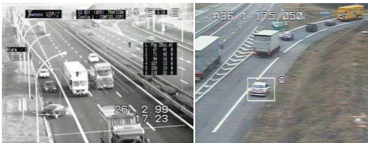
Figure 3: Wide Area Video Detection for Direct Automatic Incident Detection.
