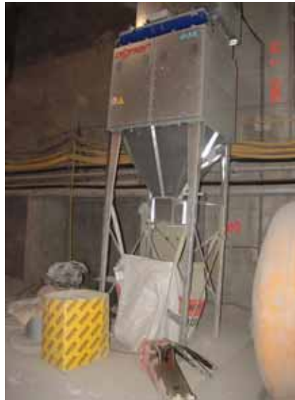
Figure 11: Dust filter of the cleaning system from EccoDust
