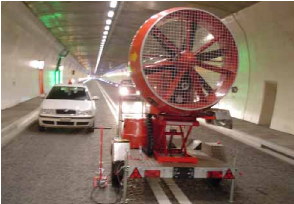
Figure 5: Mobile jet fan
