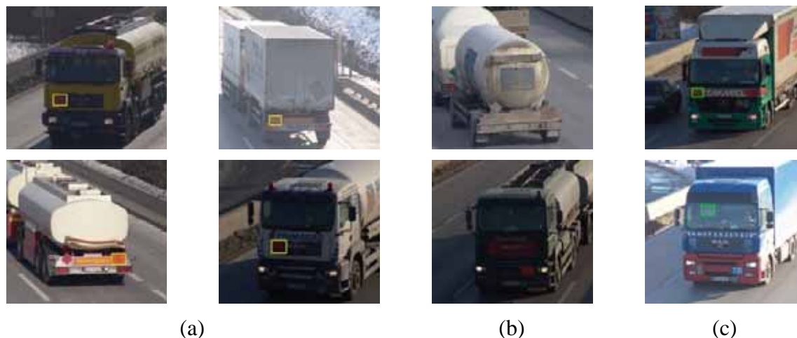
Figure 7: Illustrative detection results: (a) correctly detected plates, (b) missed plates, and (c) false positives
