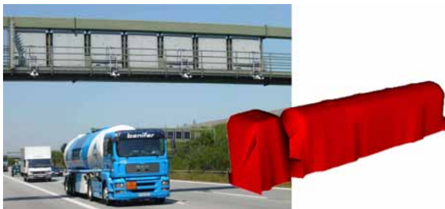
Figure 1: Overhead vehicle classification with laser scanners on the A99 motorway in Munich and the 3D model of a vehicle on the right
