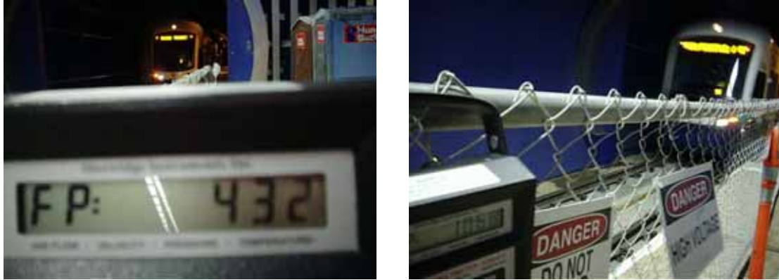
Fig. 3: Measurements taken at the platform of Beacon Hill Station (1FP = 1fpm = 0.005 m/s)
