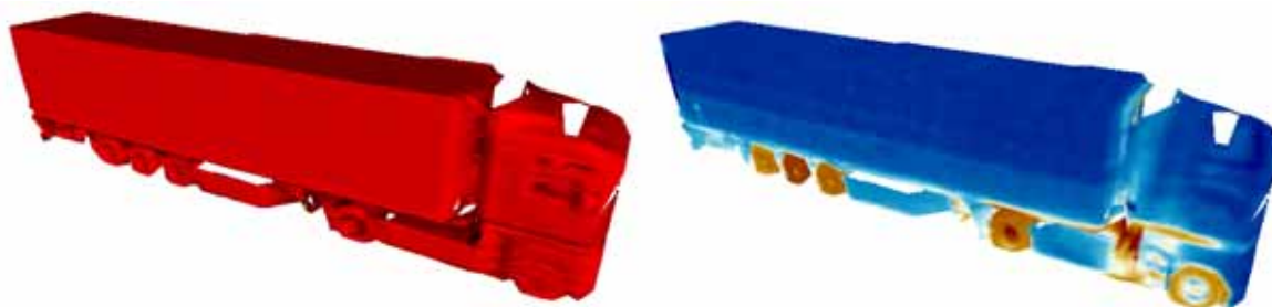
Figure 5: 3D model with the vehicle's temperature distribution on the right
