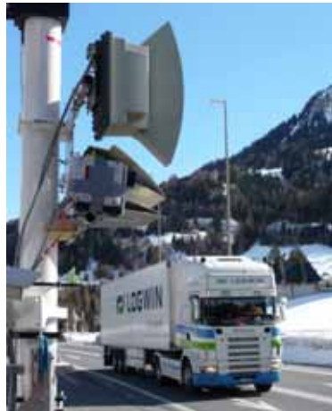
Figure 6: Vehicle hotspot detection at the Gotthard tunnel in Switzerland
