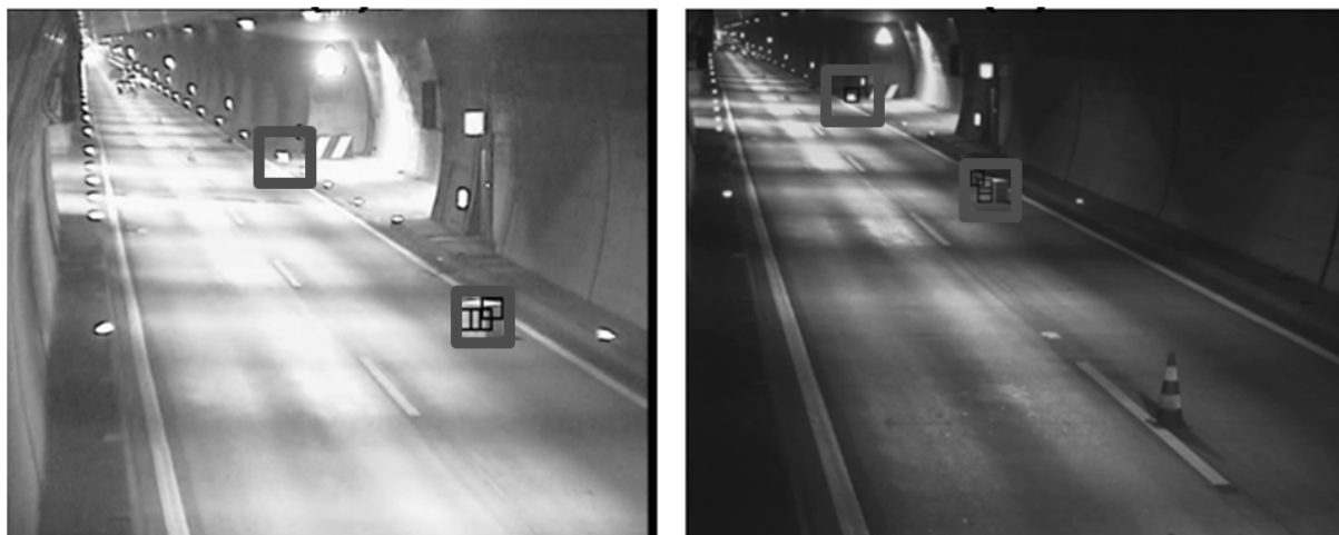
Figure 3: Lost cargo detection
