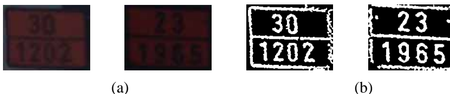
Figure 6: The original input images are insufficient as input for the OCR - a pre-processing step is required: (a) original and (b) pre-processed data
