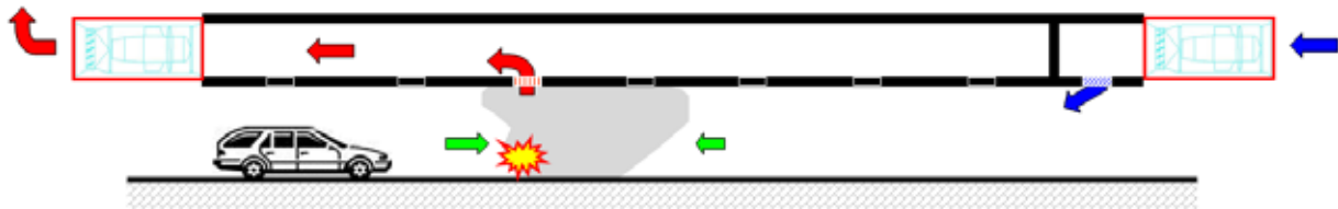
Figure 2: Sketch of a Saccardo type fresh air injection system
