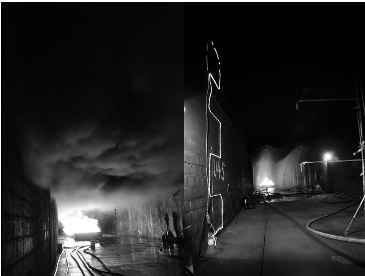
Figure 3: Smoke layer shortly after ignition and after activation of the FFFS
