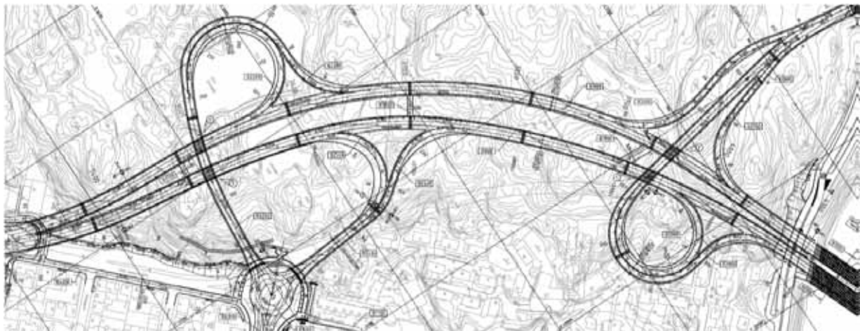
Figure 3: Tunnel with several bifurcations to and from ramps, unidirectional traffic in main tunnel but uni- and bi-directional traffic on ramps.
