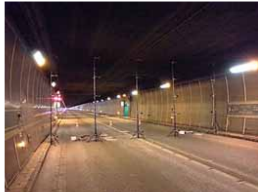
Figure 1: Scanning method (left-hand side) and anemometers mesh (right-hand side)
