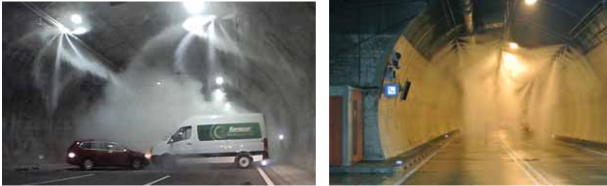
Figure 3: Car immediately after activation of the FFFS, Foam (on the left) and Water mist (on the right)
