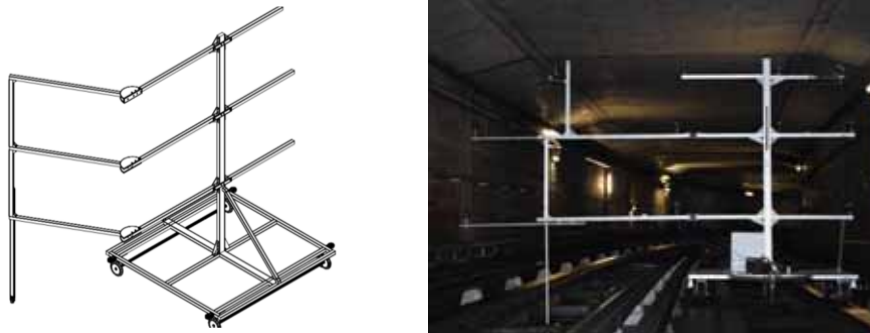
Figure 6: 3D design of the measurement foldable frame (left-hand side) and frame as-built in the tunnel (right-hand side)
