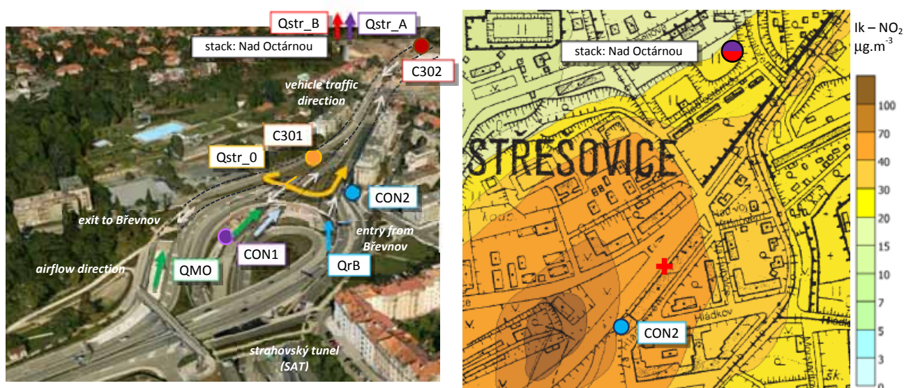
Figure 4: Measuring points by the portal, expected increase of pollution produced by the tunnel [1].
