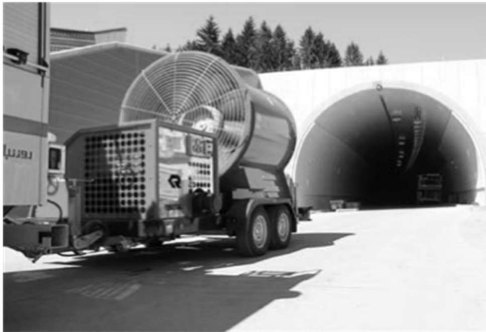
Figure 1: Location of venturi jet in front of tunnel portal
