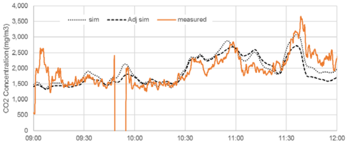
Figure 8: Comparison of calibrated CO 2 model, 26 th March 2015.
