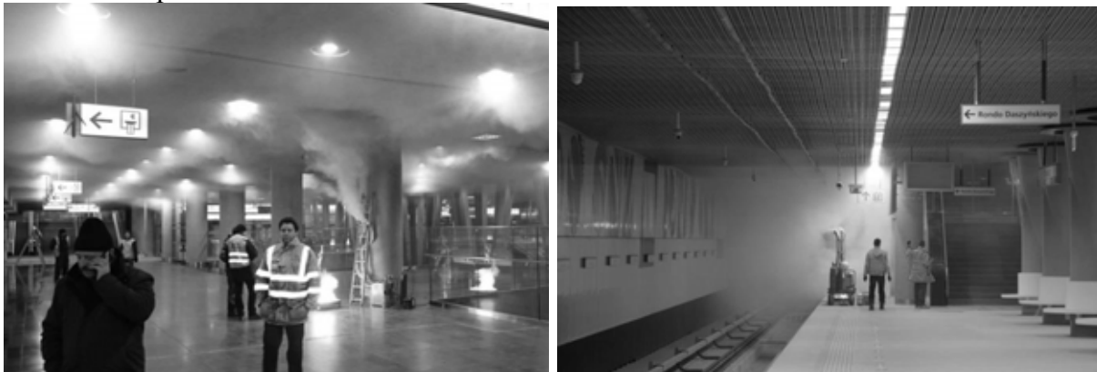
Figure 1: Hot smoke test in a Metro station, with transverse (left) and longitudinal (right) system
