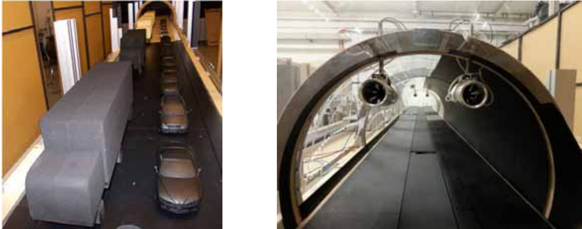
Figure 4: left: modelled congestion with standing HGV on the right lane and passenger cars on the left lane; right: Installation of jet fans in the model tunnel
