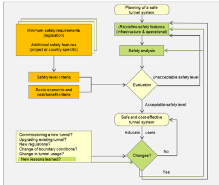
Figure 4: Integrated approach to road tunnel safety – feedback chain [10]
