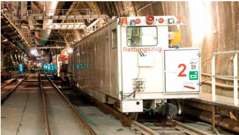
Figure 2: One of the four rescue trains at KAT2 (Source: ÖBB)
