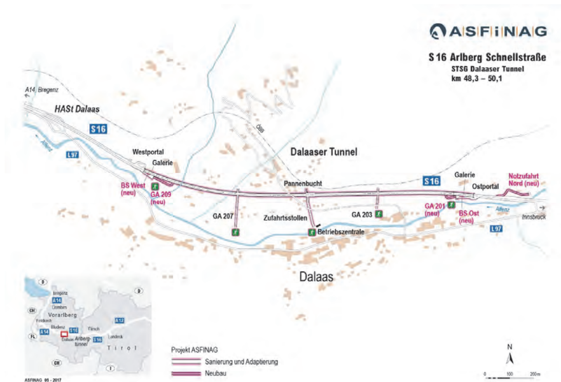
Figure 4: Location tunnel Dalaas with actual (after upgrading) situation of escape ways
