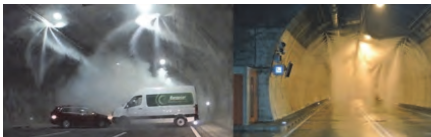
Figure 1: Experimental situation after activation of FFFS – Foam (left) – Water mist (right)
