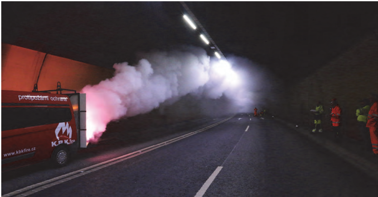
Figure 4: Moving smoke source in the Crapteig tunnel
