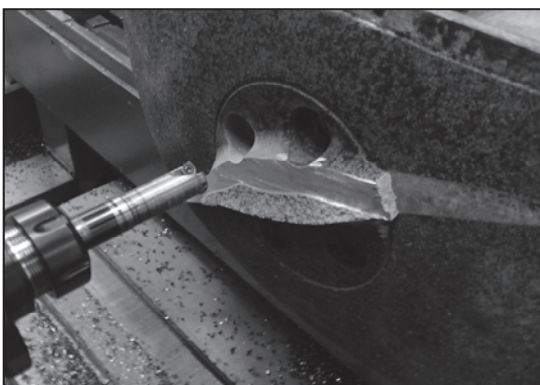
Figure 7: Mechanical removal blade
