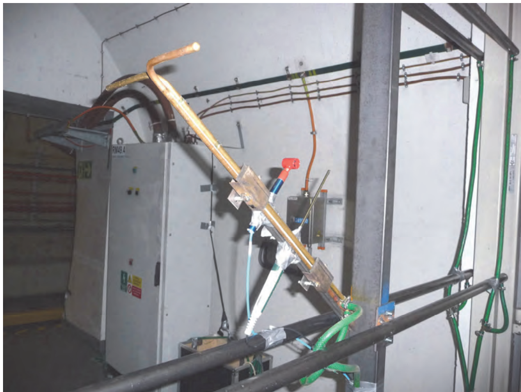
Figure 3: Arrangement of Prandtl probes for measuring static and dynamic pressure and the propeller and thermal anemometer for measuring the velocity of the air flow within the cross-section of the fire gate in cross passage
