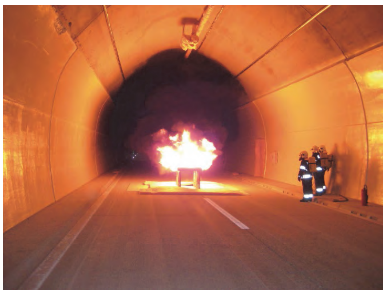
Figure 5: Underground fire test
