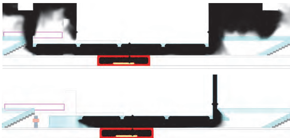
Figure 7: Comparison of smoke concentration within a station volume with a spill plume (top) and edge spill chimney installed with jet fans (bottom)
