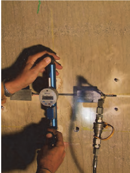
Figure 6: Slot compensation measurement to determine tunnel lining loading
